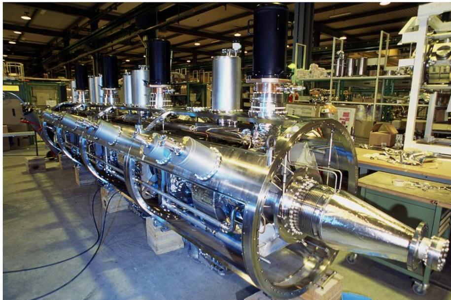
**Figure 4.2:** Four-cavity module during assembly.
